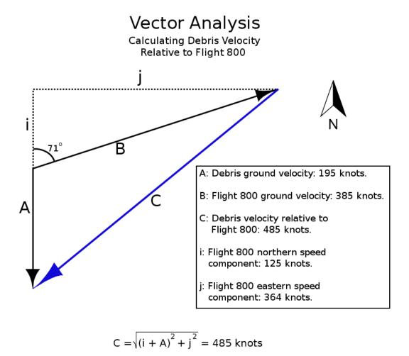
**Figure 2:** Addition of Flight 800 and debris velocity vectors. The blue line labeled **C** represents the debris' velocity relative to Flight 800. Lines **A** and **B** represent the ground velocities of the debris and Flight 800 respectively. Lines **i** and **j** represent Flight 800's northern and eastern speed components.
