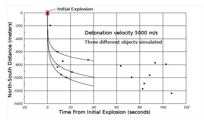
**Figure 4**: Three ballistics curves fit to north-south position vs. time from the Islip and White Plains radar sites. This plot only shows the north-south distances and speeds. Flight 800 was heading ENE at 385 knots. The small blue squares are a composite of Islip and White Plains FAA radar returns.
