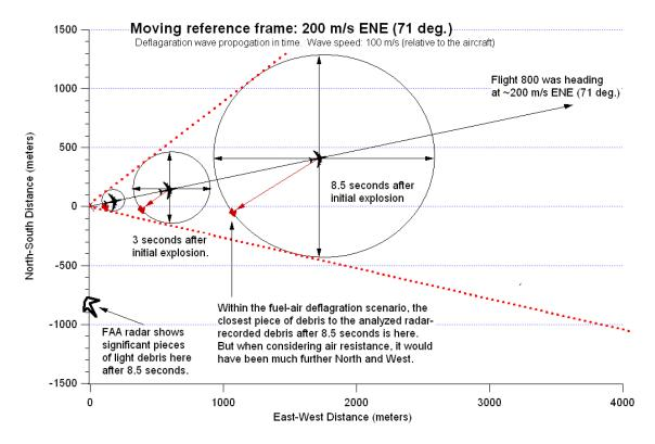
**Figure 3:** Maximum deflagration wave expansion at three points in time in TWA Flight 800's reference frame. Air resistance is neglected outside the aircraft to provide a best-case scenario for the NTSB's crash sequence. The red arrows point to hypothetical debris ejected by the deflagration. The 747 icons are not to scale.
